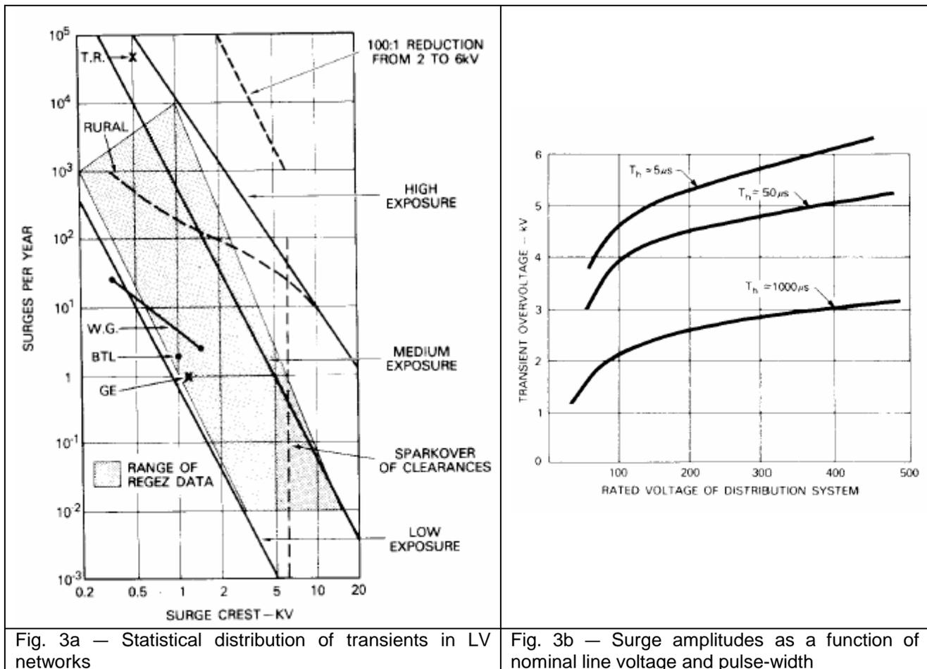
Fig. 3a — Statistical distribution of transients in LV networks
