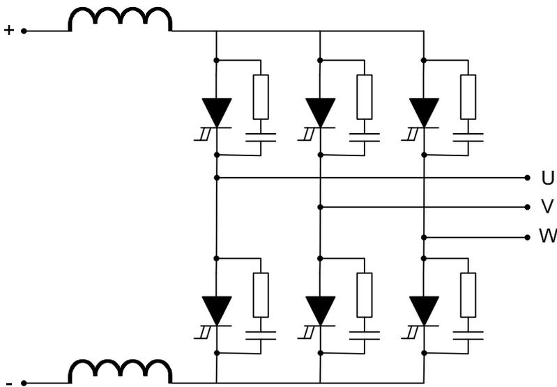
Fig. 6 – Current Source Inverter with reverse blocking IGCTs
