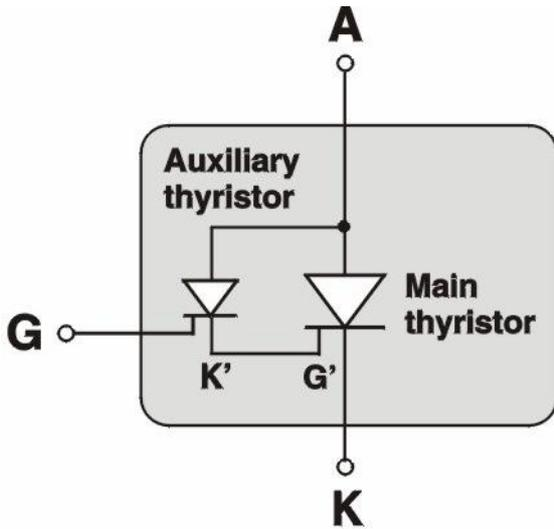
Fig. 2 — Basic principle of the amplifying gate
