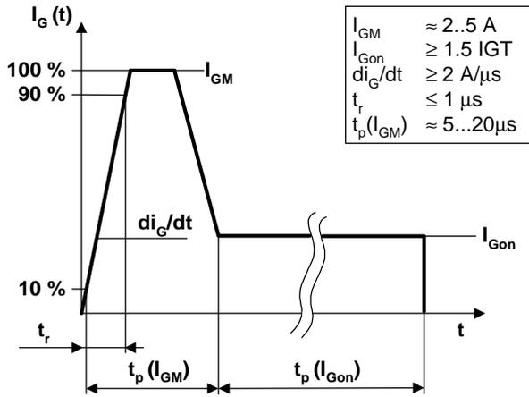
Fig. 6 — Recommended gate-pulse for ABB phase-control thyristors
