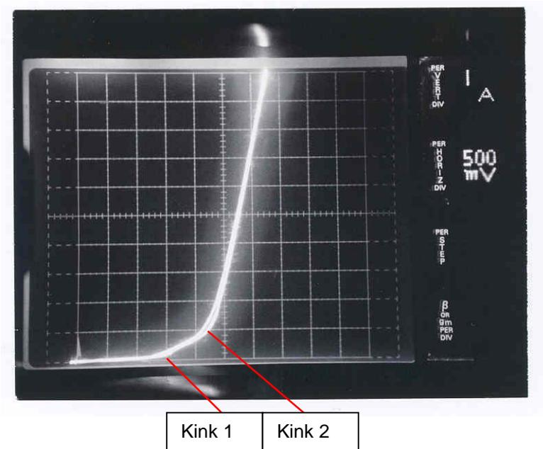
Fig. 5 — Amplifying gate characteristic of thyristor 5STP 26N6500
