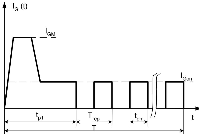
Fig. 9 — Example of a picket-fence gate-pulse train
