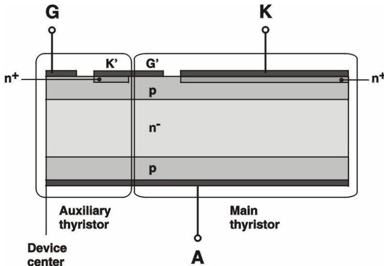
Fig. 3 — Lateral integration of the amplifying gate
