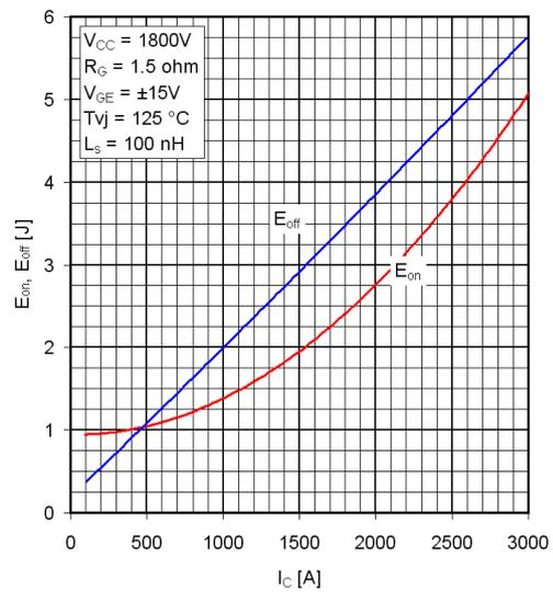
Figure 7: 3.3kV/1200A SPT<sup>+</sup> IGBT HiPak  $E_{on}$  and  $E_{off}$  vs.  $I_c$  losses curves
