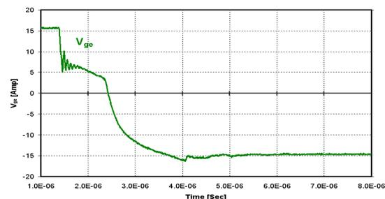
Figure 11: 3.3kV/1200A SPT<sup>+</sup> IGBT HiPak turn-off SOA waveforms at 125°C
