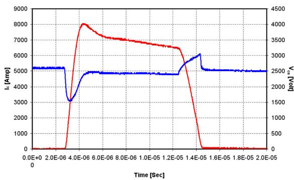
Figure 16: 3.3kV/1200A SPT<sup>+</sup> IGBT HiPak SCSEA waveforms at 125°C
