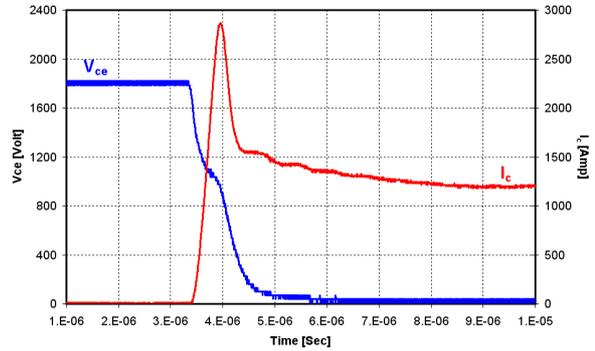
Figure 6: 3.3kV/1200A SPT<sup>+</sup> IGBT HiPak turn-on waveforms at 125°C
