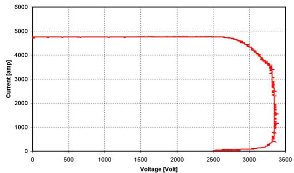
Figure 14: 3.3kV/1200A SPT<sup>+</sup> IGBT HiPak I/V square RBSOA curve.
