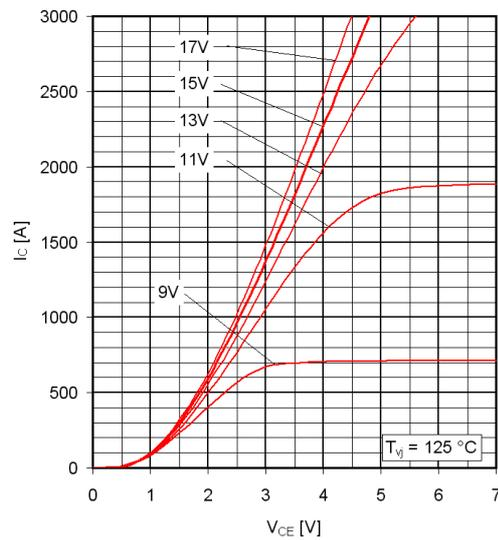
Figure 3: 3.3kV/1200A SPT<sup>+</sup> IGBT HiPak output characteristics at 125°C
