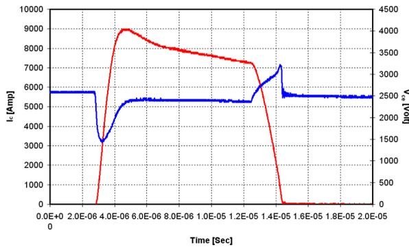
Figure 15: 3.3kV/1200A SPT<sup>+</sup> IGBT HiPak SCSEA waveforms at 25°C
