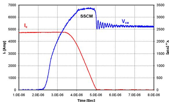
Figure 13: 3.3kV/1200A SPT<sup>+</sup> IGBT HiPak turn-off SOA waveforms at 125°C with “SSCM”
