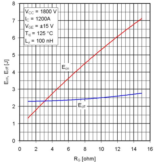
Figure 8: 3.3kV/1200A SPT<sup>+</sup> IGBT HiPak  $E_{on}$  and  $E_{off}$  vs.  $R_g$  losses curves
