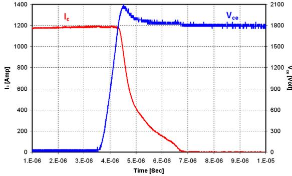
Figure 5: 3.3kV/1200A SPT<sup>+</sup> IGBT HiPak turn-off waveforms at 125°C
