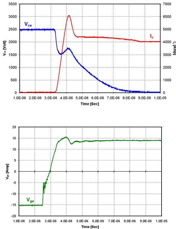
Figure 12: 3.3kV/1200A SPT<sup>+</sup> IGBT HiPak turn-on SOA waveforms at 125°C
