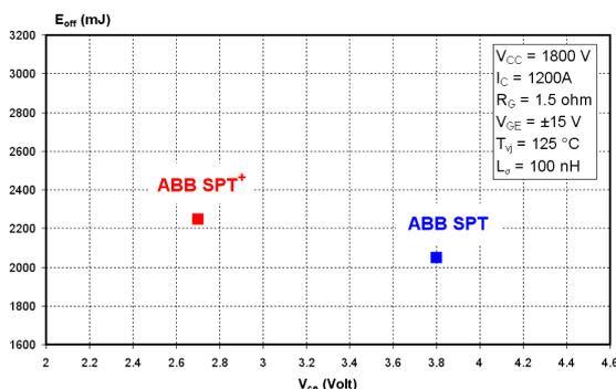
Figure 1: New 3300V/1200A SPT<sup>+</sup> IGBT HiPak technology benchmark
