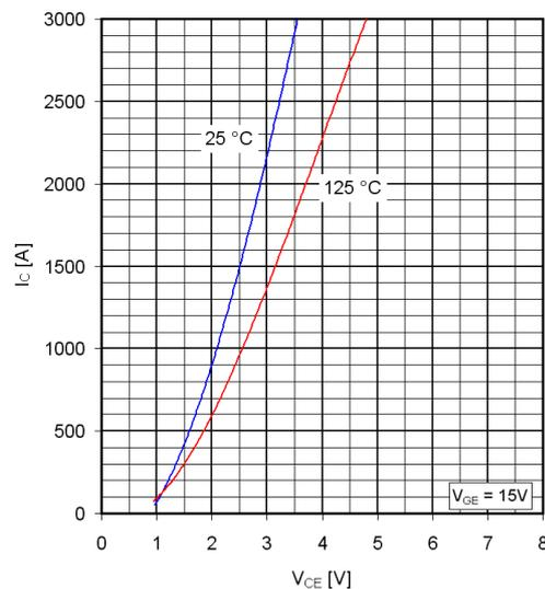
Figure 4: 3.3kV/1200A SPT<sup>+</sup> IGBT HiPak on-state characteristics at 25°C and 125°C
