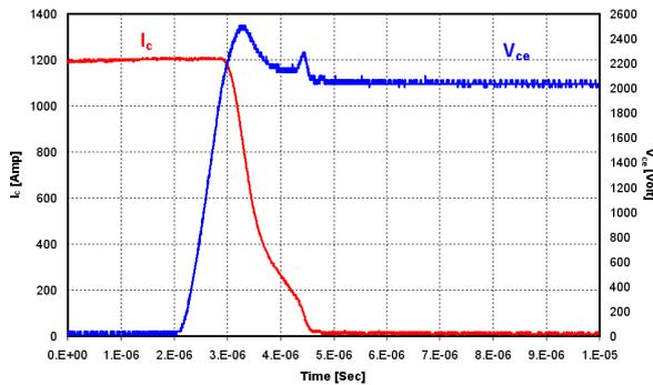
Figure 9: 3.3kV/1200A SPT<sup>+</sup> IGBT HiPak turn-off waveforms at 125°C
