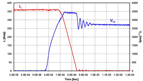
Figure 10: 3.3kV/50A SPT<sup>+</sup> IGBT Chip turn-off SOA waveforms at 125°C with "SSCM"
