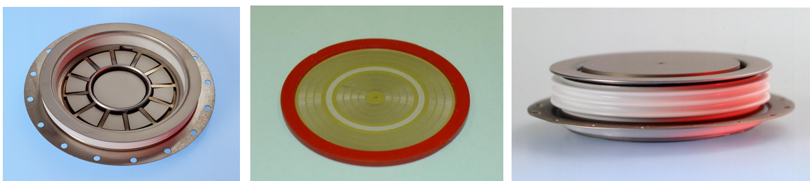
Figure 2. Low Inductive Housing, GTO-Like wafer and Complete Device
