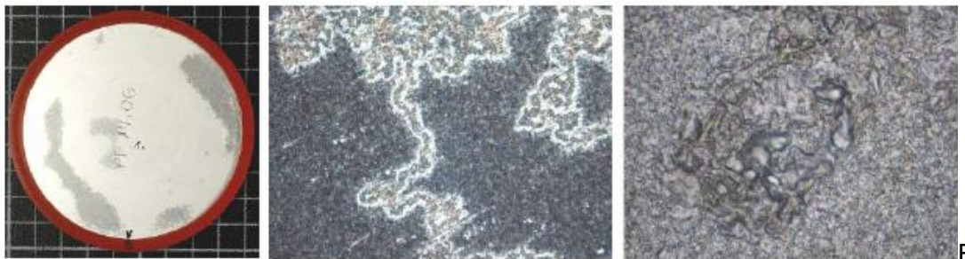
Figure 9: Anode side of wafer with partly melted aluminium contact layer. The middle picture is enlarged 45x, right picture 440x
