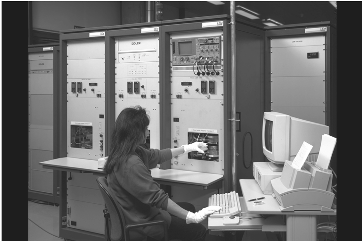
Fig. 3 Static and Dynamic Diode Tester up to 6 kV and 6 kA per Table 2
