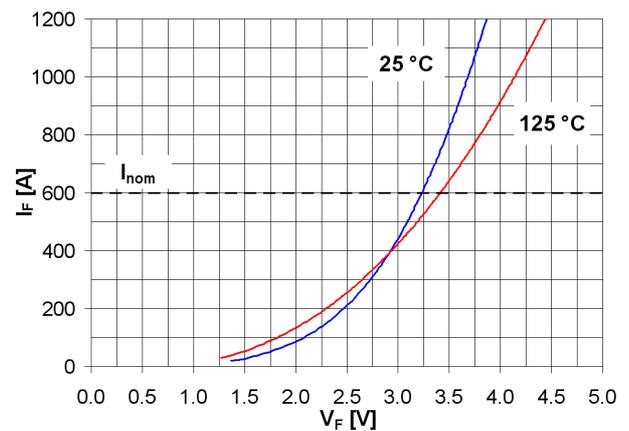
(b) Forward characteristics of the 6.5kV SPT-diode
