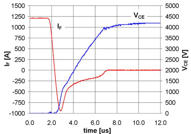
Figure 11. 6500V/600A HV-HiPak™ diode reverse recovery characteristics under SOA stress. V<sub>CC</sub> = 4400V, I<sub>F</sub> = 1200A, R<sub>Gon</sub> = 3.9Ω, L<sub>σ</sub> = 300nH, T<sub>j</sub> = 125 °C
