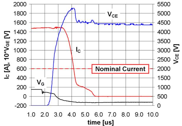
Figure 10. 6500V/600A HV-HiPak™ IGBT turn-off characteristics under high SOA conditions. V<sub>CC</sub> = 4400V, I<sub>C</sub> = 1500A, R<sub>Goff</sub> = 1.5Ω, L<sub>σ</sub> = 300nH, T<sub>j</sub> = 125 °C.
