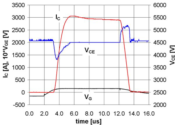
Figure 12. 6500V/600A HV-HiPak™ SCSOA characteristics.
