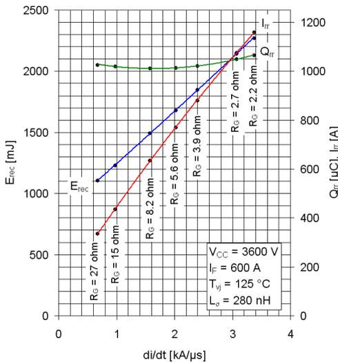
Figure 9. 6.5kV/600A HV-HiPak™ E<sub>rec</sub>, I<sub>rr</sub>, Q<sub>rr</sub> vs. di/dt curves.
