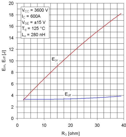
Figure 8. 6.5kV/600A HV-HiPak™ E<sub>on</sub> and E<sub>off</sub> vs. R<sub>g</sub> curves.
