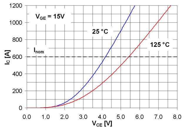
(a) Forward characteristics of the 6.5kV SPT-IGBT
