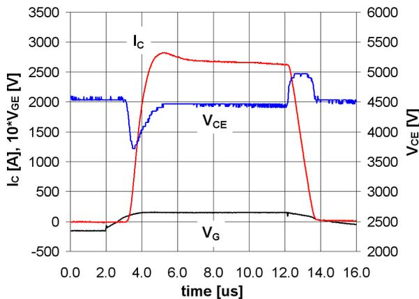
Figure 13. 6500V/600A HV-HiPak™ SCSOA characteristics.
