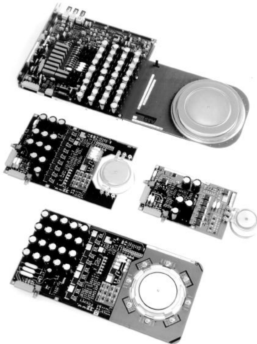
Fig. 5: Photograph of the reverse conducting IGCTs
