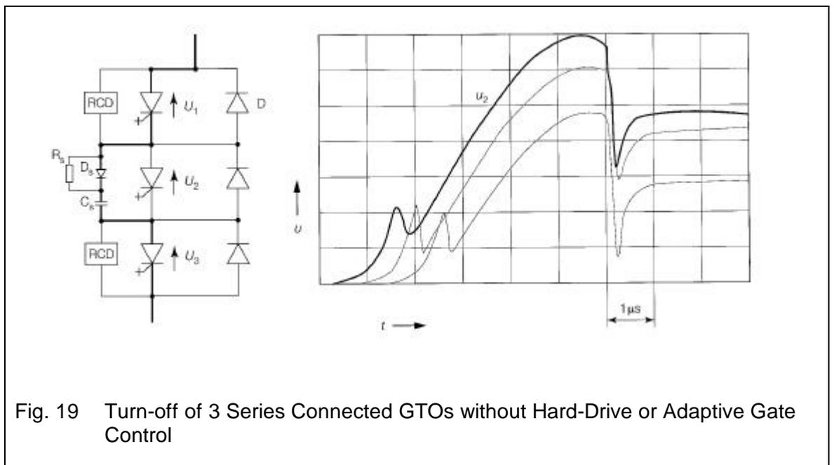
Fig. 19 Turn-off of 3 Series Connected GTOs without Hard-Drive or Adaptive Gate Control
