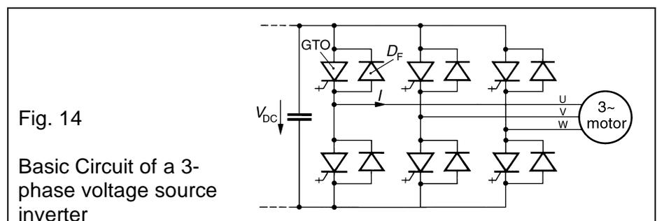
Current and voltage waveforms at the output of an inverter are illustrated in Fig. 15. Only the instantaneous values  $+V_{DC}$ , 0 and  $-V_{DC}$  can be applied across the two motor terminals, and these are alternately switched by the GTOs and diodes.
