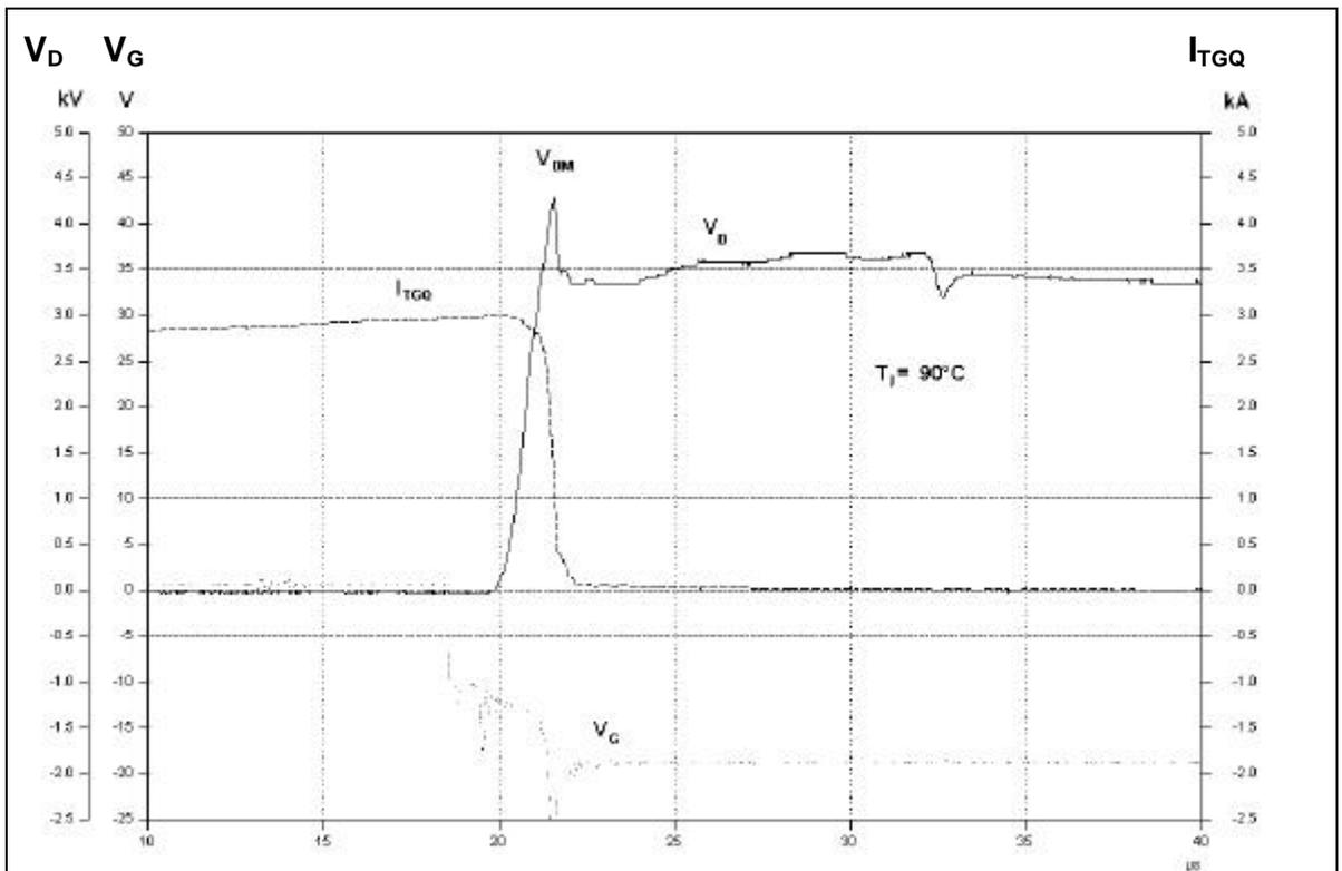
Fig. 7 Snubberless Turn-off of a 3 kA/4.5 kV GCT
