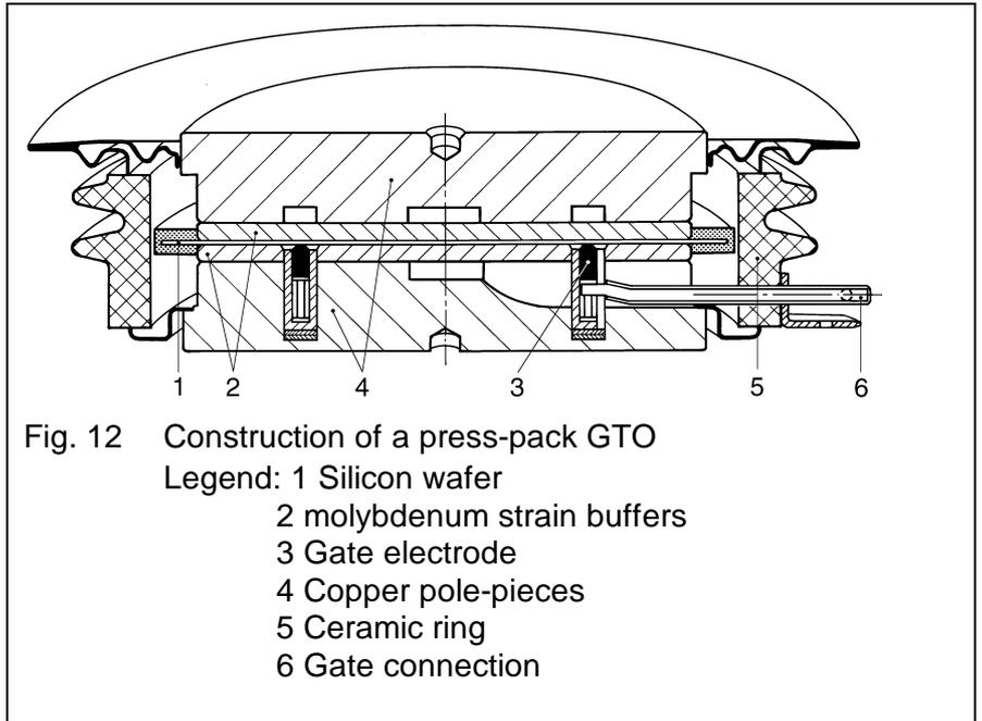
The gate electrode is recessed in the copper pole-piece on the cathode side, and electrically isolated. For small wafer diameters, a central gate contact is sufficient, whereas for GTOs with high turn-off currents above about 2000 A, the gate electrode is, in most cases, annular thus halving the distance between the gate contact-to-wafer and the most remote cathode fingers. Fig. 13 depicts various wafer designs.
