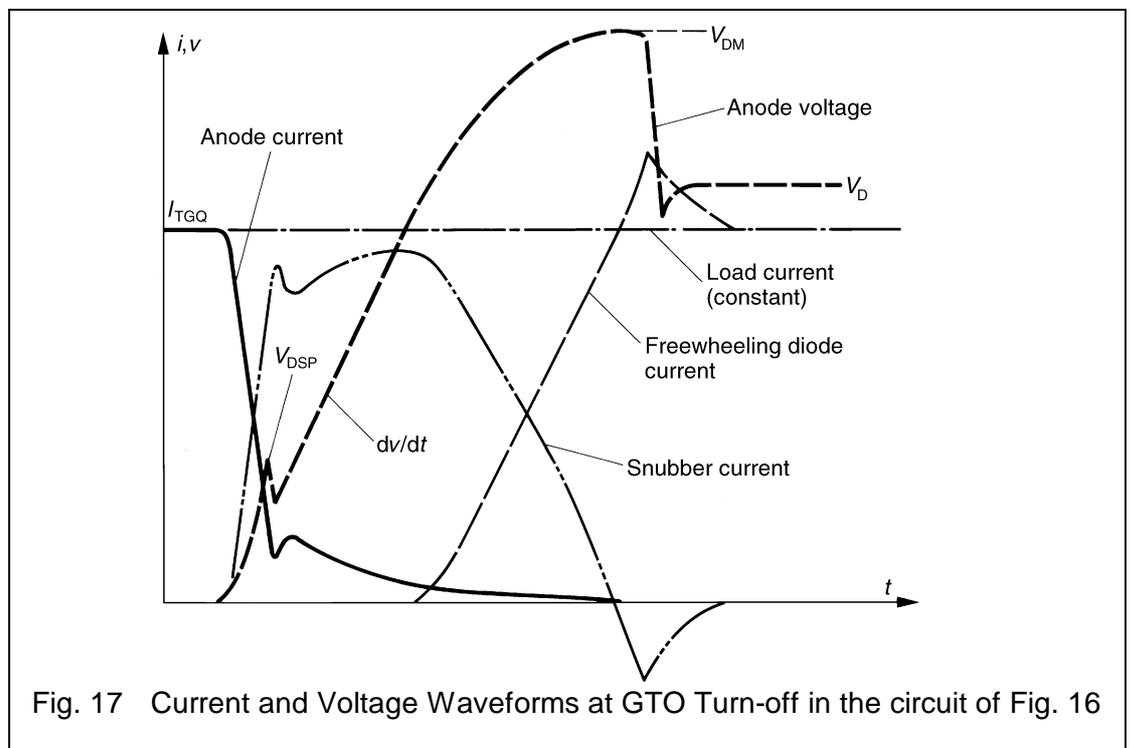
Fig. 17 Current and Voltage Waveforms at GTO Turn-off in the circuit of Fig. 16
