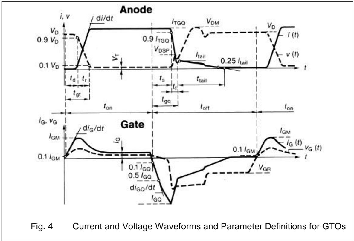
Fig. 4 Current and Voltage Waveforms and Parameter Definitions for GTOs
